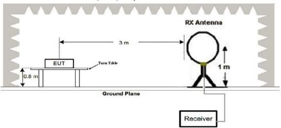
(2) Radiated Emission Test-Up Frequency 30MHz~1GHz
