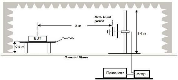
(3) Radiated Emission Test-Up Frequency Above 1GHz
