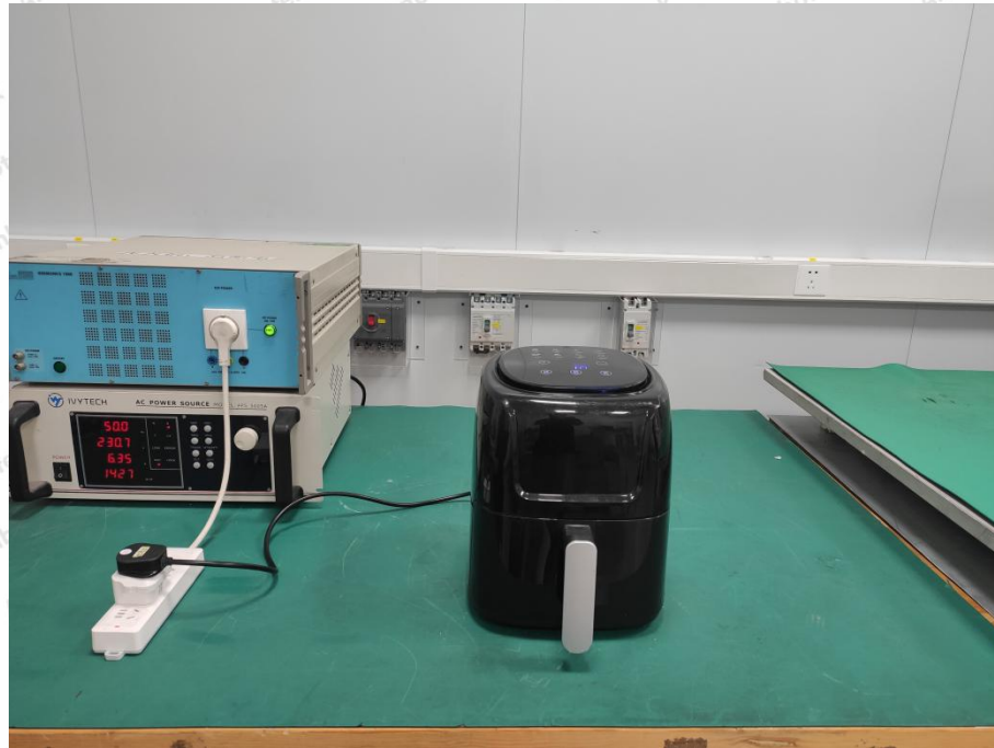
Photo of Harmonic Current And Flicker Test
