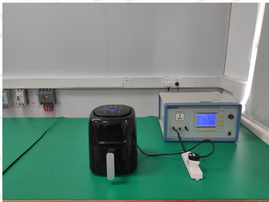
Photo of Voltage Dips and Interruptions Immunity Test
