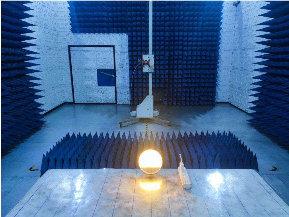
Radiated emissions at frequencies above 1 GHz
